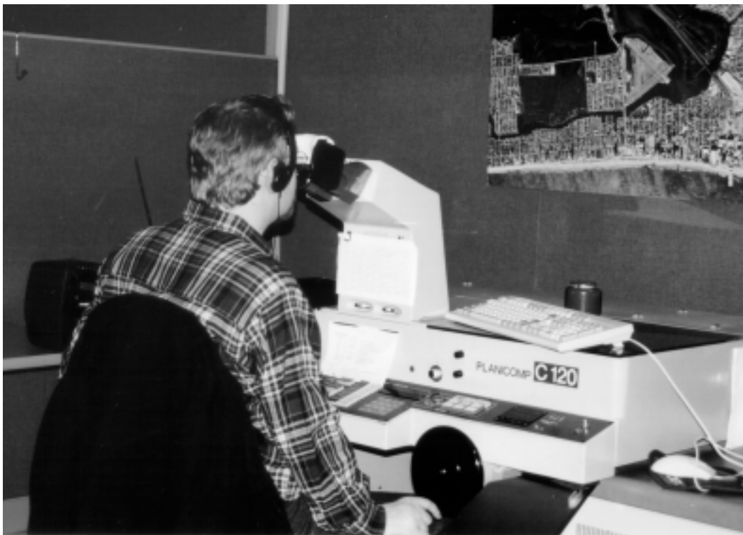
Figure 9-1. Typical analytical stereoplotter (courtesy of Surdex Corporation)
