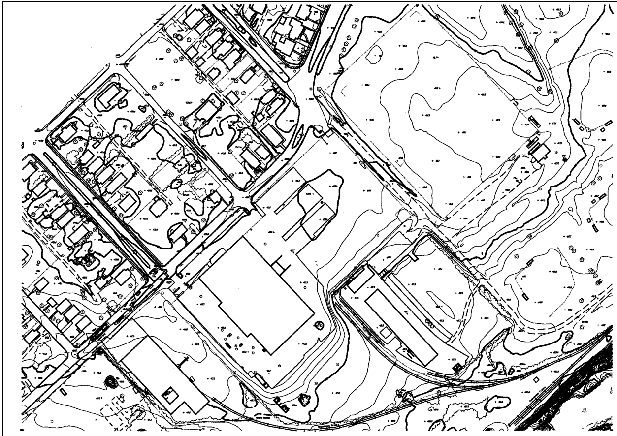
Figure 9-4. Typical planimetric data set with contours (courtesy of Barton Aerial Technology)
